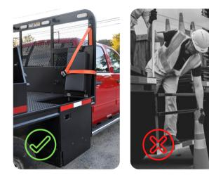
Box positioning keeps workers more shielded by the bed from collision and effectively **increasing effective visual and verbal communication** between workers and the driver.
